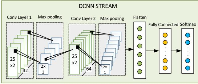
Fig. 2: The deep convolution neural network stream.
